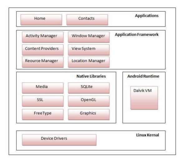
At the core of the Android platform is a Linux kernel responsible for device drivers, resource access, power management, and other OS duties. The supplied device
